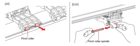
4 Mount new pinch rollers, and secure them using the O-ring.
